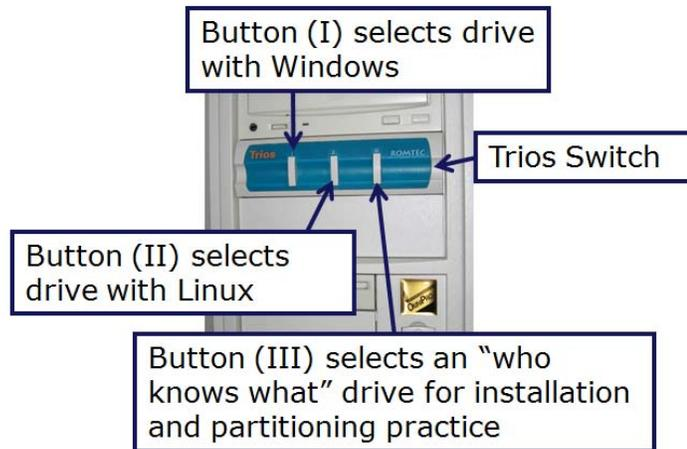
There are some older PC's in room 2504 with Trios switches. The Trios switch allows selecting one of three hard drives. The second hard drive has Linux installed. While the computer is off press the second Trios button in. The PC will power up and run Linux.
