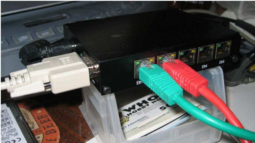
*Assemble your own Linux based Router. This one has five Ethernet interfaces and uses 6.4 watts of power.*
