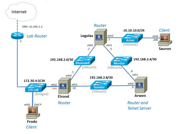
Lab 4 NETWORK DIAGRAM: Each switch above is really a virtual network. The white labels are the names used in the VLab pods (VMware ESXi/vSphere) and the gray labels in parenthesis are the names used on the workstations in the CIS Lab (VMware Workstation).
