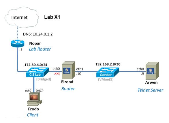
Lab X1 NETWORK DIAGRAM: Each switch above is really a virtual network. The white labels are the names used in the VLab pods (VMware ESXi/vSphere) and the gray labels in parenthesis are the names used in on the workstations in the CIS Lab (VMware Workstation).
