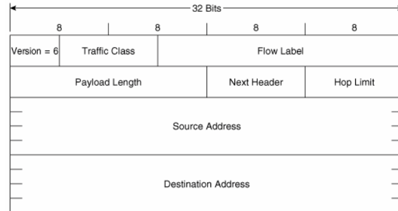
Figure 2-5. The IPv6 packet header.
