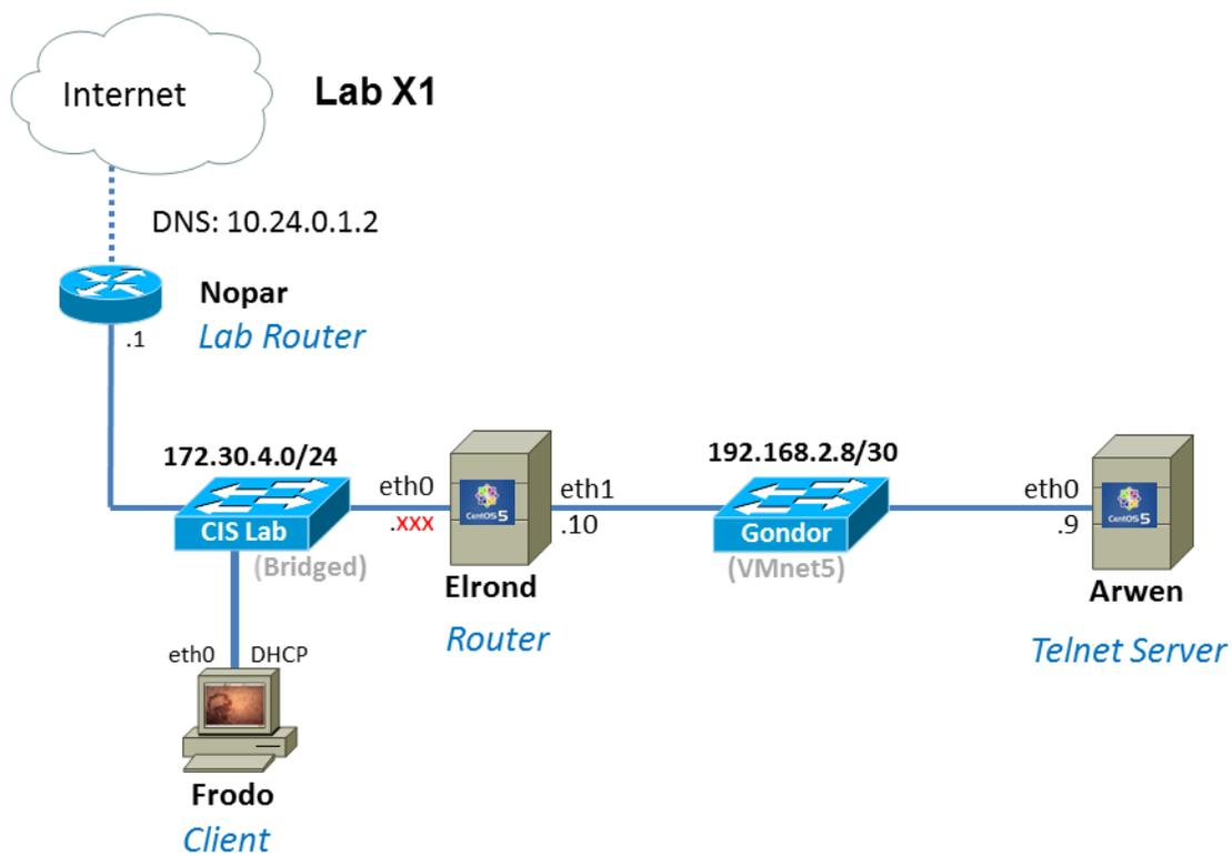
Lab X1 NETWORK DIAGRAM: Each switch above is really a virtual network. The white labels are the names used in the VLab pods (VMware ESXi/vSphere) and the gray labels in parenthesis are the names used in on the workstations in the CIS Lab (VMware Workstation).
