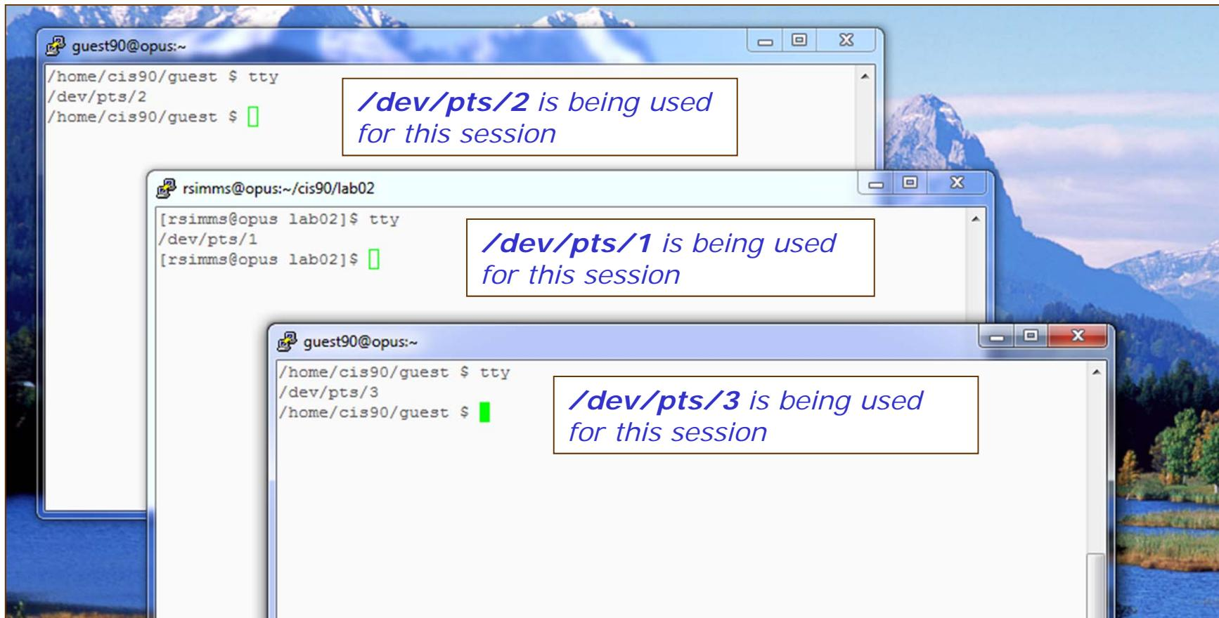
*Use the **tty** command to identify the **terminal device** being used for a session*
