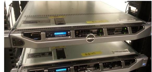
*The CIS 90 systems, e.g. Opus and Sun-Hwa, are virtual machines hosted on physical servers in the CIS Lab*
