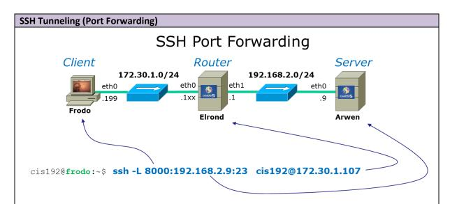
Any connection made to port 8000 on Frodo will get forwarded to port 23 on Arwen via Elrond. The portion of the connection between Frodo and Elrond will be encrypted
