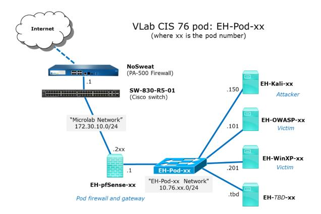
Each pod has been populated with an initial set of VMs but they have not been fully configured yet. In the diagram above the "xx" represents the pod number. We need to configure the VMs in your pod so they are cabled into your own pod network, have unique hostnames and IP addresses and some backup snapshots made.
