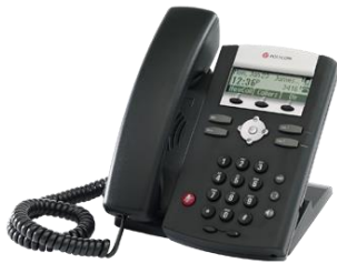
SIP phone is connected using standard LAN cable
