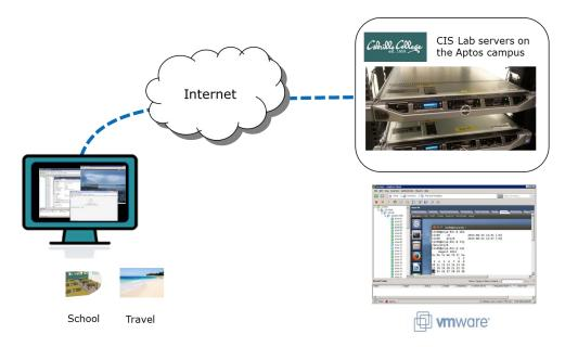
Students remotely connect to the main CIS VLab server on campus using an RDP client. RDP is already built into Windows but must be added as third party software to a Mac. Once connected the VMware vSphere Client is automatically run which then enables a student to select one of the virtual machines to use.
